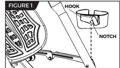
Alternatively, the Storage Caddy can be installed on the **RIGHT, REAR** side of the A-frame.
