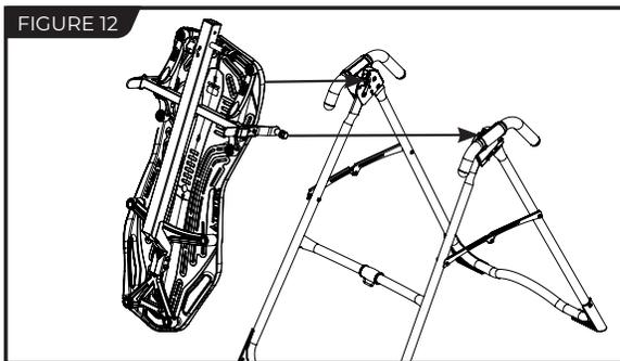
TIP: You may need to push outward on the Hinge Plate in order for the second Pivot Pin to lock in place.
